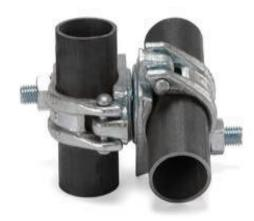
These are Heavy duty Swivel couplers manufactured using Drop Forged process. Used for connecting two scaffold tubes at any angle to each other: confirming to IS-2750/BS-1139.
