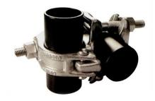
These are Heavy duty Right angle couplers manufactured using Drop Forged process and known as Double Coupler also. Used for connecting two scaffold tubes at right angle to each other: confirming to IS-2750/BS-1139.
