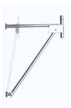
This item is used for providing support to decking or form work at edges. This frame has ledger blades to be fitted into cups of cuplock standards at one end & with provision for accepting jacks in three position at the other end at 1.2m, 1.25m and 1.3m from center line of the standard.
