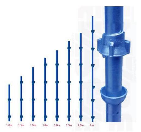
Made out of 40mm, N.B. 'M' or 'H' Tubes confirming to I.S. 1161/I.S. 1239 grade - YST 210/240 with provision of cups at 500mm / 1000.. c/c
