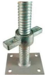
Made out of 150x150x6 mm or 150x150x5mm flat 7 M.S> Bar for 32mm or 36mm dia. Rolled Threading with adjustment of 225mm or 350mm or 450mm. These base plates give stability to scaffolding with desired adjustment at the base. These are also available with Rolled Threading in Hollow Tubes.
